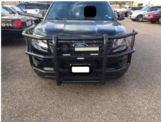
16. Item # 16 – (New) Front bumpers with wing guards (Go Industries bumper and wings or similar).
